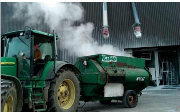
Figure 2: Homogenisation of manure and lime outside (United Kingdom)
